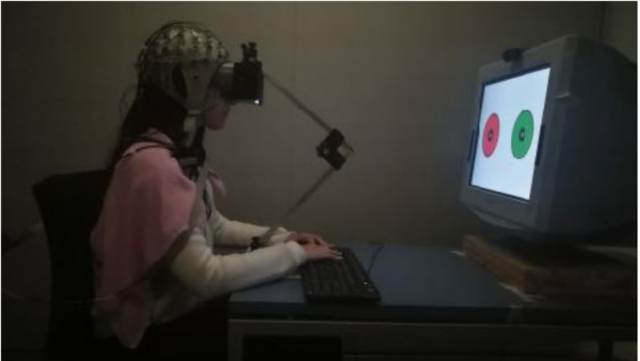
Figure 3. A participant performs the Binocular Rivalry task with the EEG configuration
