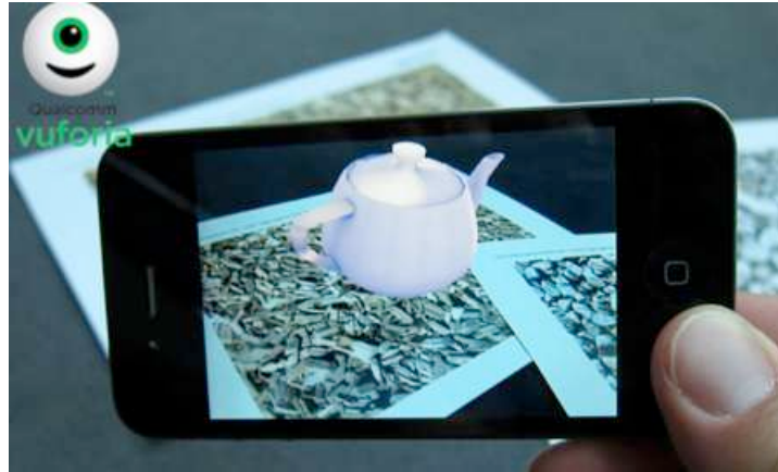
Figure 4 – Vuforia AR platform displaying a 3D model of a teapot on top of a marker
