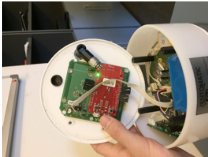
FIGURE 11. DETAIL ON THE CONFIGURATION OF THE TRAP (ONCE THE RED BUTTON IS PRESSED, PRESS THE RIGHT BUTTON AND WAIT UNTIL THE GREEN LED IS ON)
