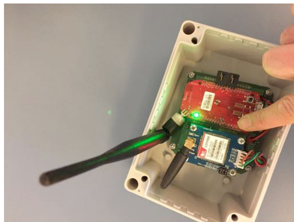
FIGURE 10. DETAIL ON THE SECOND STEP TO CONFIGURE THE GATEWAY (LEFT BUTTON AND WAIT UNTIL THE GREEN LED IS ON)
