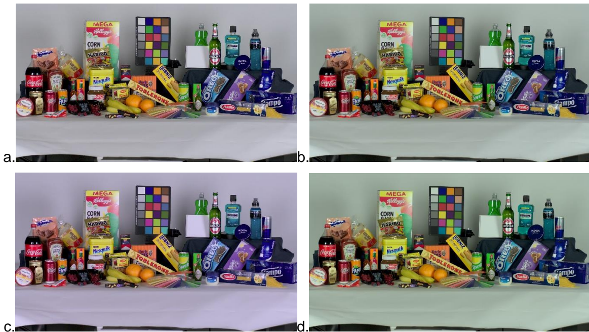
Figure 5. sRGB renderings of images shifted to make a metameric match between a Sony BVM-CRT and IMAX laser projector for a set of observers . Panel a. shows the sRGB source image, and the matches for observers 3 (panel b.), 7 (panel c.), and 10 (panel d.) are shown. Test image provided by Arri Camera Systems.
