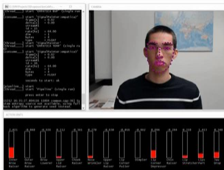
Figure 9: Real-time calculation of ActionUnits. These features offer the possibility to classify emotions based on the facial expression. AU's such as LipCornerDepressor , CheekRaiser or UpperLipRaiser are especially well suited to detect states of valence.
