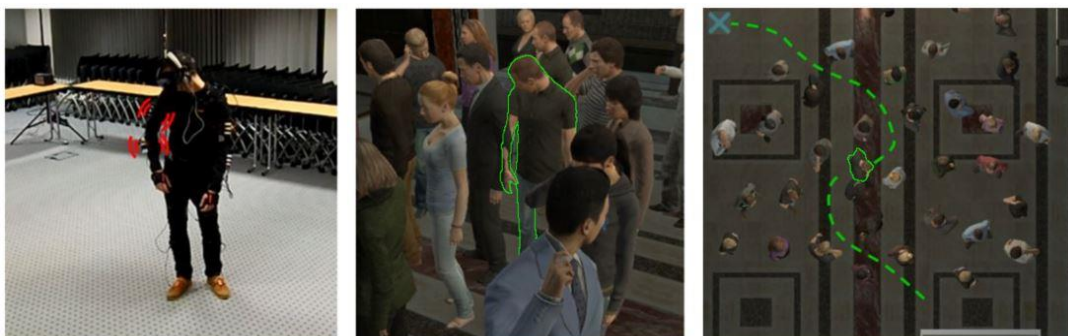
Figure 15 - We investigated the influence of rendering physical contacts while navigating in a virtual crowd. Participants wore a Xsens motion capture suit, wearable haptics armbands, and a wide-field-of-view HMD.
