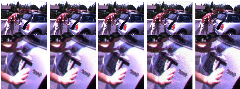
Figure : First column: Original frame. Second Column: noisy frame with \sigma = 10 . Third Column: Denoised frame with \sigma = 10 . Fourth Column: noisy frame with \sigma = 20 . Fifth Column: Denoised frame with \sigma = 20 .
