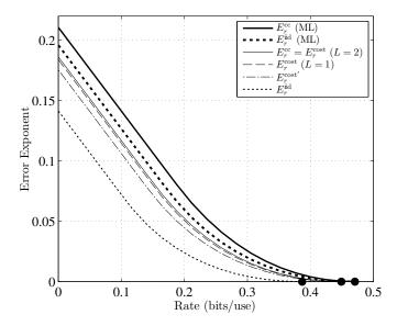
Figure 1. Error exponents for the channel defined in (56) with  $\delta_0=0.01$ ,  $\delta_1=0.05$ ,  $\delta_2=0.25$  and Q=(0.1,0.3,0.6). The mismatched decoder uses the minimum Hamming distance metric. The corresponding achievable rates  $I_{\rm GMI}(Q)$ ,  $I_{\rm LM}(Q)$  and I(X;Y) are respectively marked on the horizontal axis.
