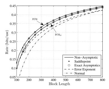
Figure 3. Rate required to achieve a target error probability  $\epsilon$  for the channel defined in (56) with ML decoding. The parameters are  $\epsilon=10^{-8}$ ,  $\delta_0=\delta_1=\delta_2=\delta=0.1$  and  $Q=(\frac{1}{3},\frac{1}{3},\frac{1}{3})$ .
