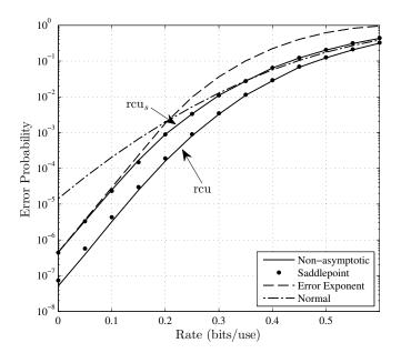
Figure 2. i.i.d. random-coding bounds for the channel defined in (56) with minimum Hamming distance decoding. The parameters are  $n=60, \, \delta_0=0.01, \, \delta_1=0.05, \, \delta_2=0.25$  and  $Q=(\frac{1}{3},\frac{1}{3},\frac{1}{3}).$
