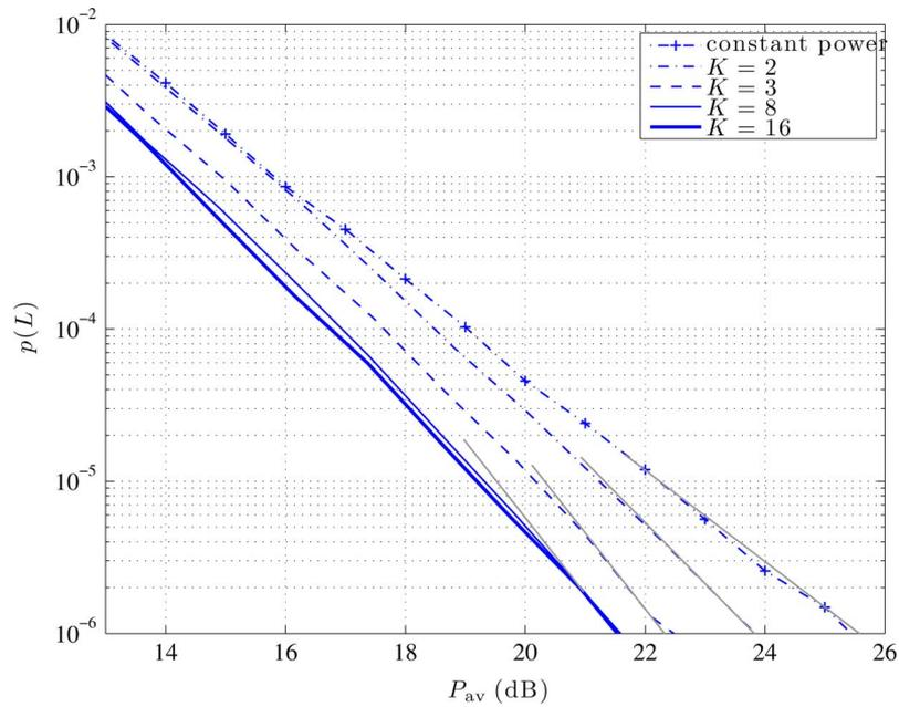
Fig. 5. Outage performance of ARQ transmission schemes for a 16-QAM input block-fading channel with  $L = 2$ ,  $N_t = N_r = 1$ ,  $B = 2$ ,  $R = 3.5$ . The gray lines represent the optimal asymptotic slope.
