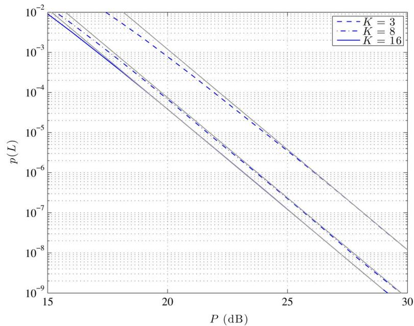
Fig. 7. Upper bound on outage performance of ARQ transmission schemes using 16-QAM constellation over the block-fading channel with  $L = 2, N_t = N_r = 1, B = 2, R = 3.5$  and  $K = 3, 8, 16$ . The gray lines represent the asymptotic bound with diversity 5.
