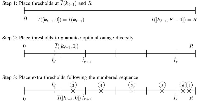
Fig. 4. Example of feedback threshold design ( $K = 12$ ).
