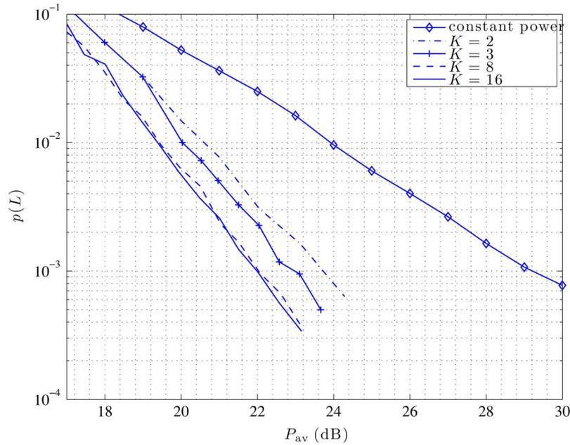
Fig. 6. Outage performance of ARQ transmission using the 16-QAM input constellation over the block-fading channel with  $L = 2, N_t = 2, N_r = 1, B = 1, R = 7.5$ . Systems with constant transmit power, and systems employing power adaptation with  $K = 2, 3, 8, 16$  are considered.
