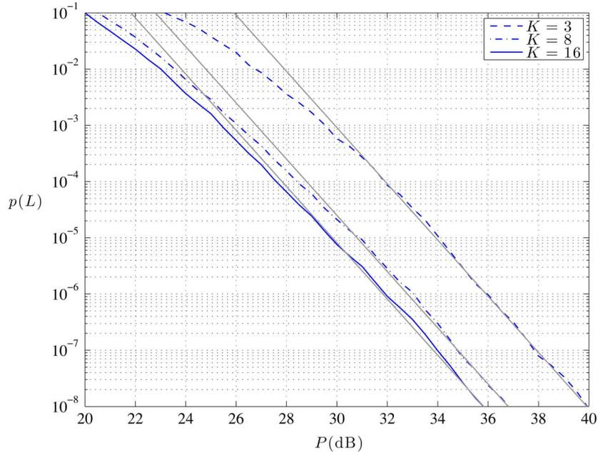
Fig. 8. Upper bound on outage performance of ARQ transmission using 16-QAM input constellations over the block-fading channel with  $L = 2$ ,  $N_t = 2$ ,  $N_r = 1$ ,  $B = 1$ ,  $R = 7.5$  and  $K = 3, 8, 16$ . The gray lines represent the asymptotic bound with diversity 5.
